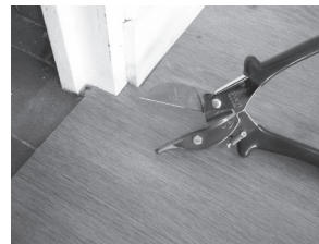
Mitre shears Reference: Romus: 93401 / Janser: 237 530 000 For cutting around door frame bases, areas which are difficult to access.
